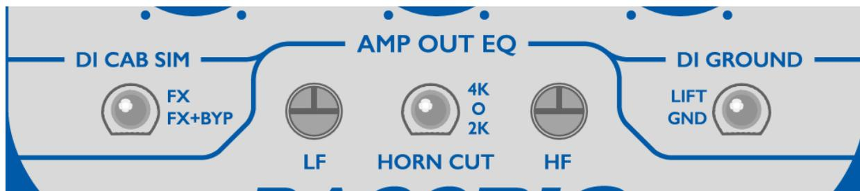
The post-drive AMP OUT EQ ensures compatibility with a wide range of amps and cabs. Instead of compromising your amp's tone controls to suit the BASSRIG, set your amp for your preferred clean sound then use the EQ controls to adjust the pedal's output accordingly (see tables on page 8).
